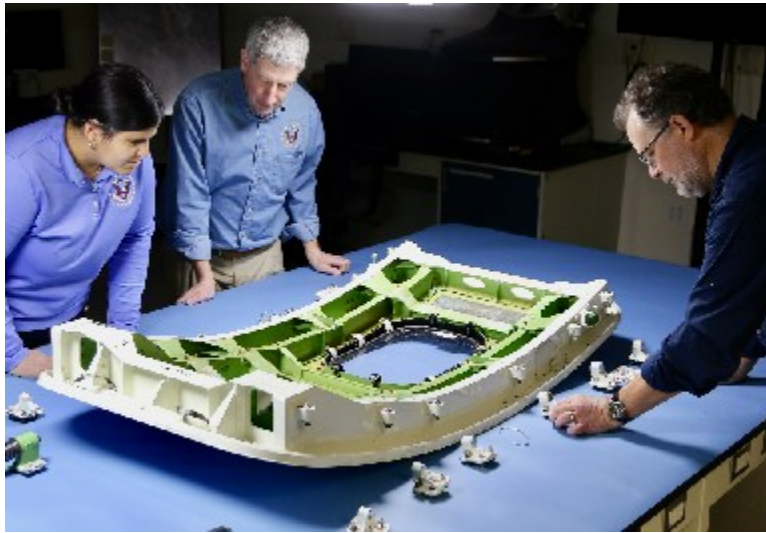
NTSB investigators examine the door plug from Alaska Airlines flight 1282, a Boeing 737-9 MAX. NTSB
