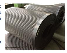
JMA vacuum filter belt separates the goods from the liquid by acid or leaching or by rinsing the liquid out. As long as the fillet belt continuously circulating, with the help of gravity and the vacuum generated by the vacuum box below, the separated liquid passes through the holes of the belt and gathers into the vacuum box, at the same time the dry goods is taken away on the filter belt.
