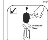
ALWAYS USE A PROTECTIVE PIECE OF WOOD (NOT INCLUDED) BEFORE HAMMERING THE TOP OF THE METAL SPIKE.
