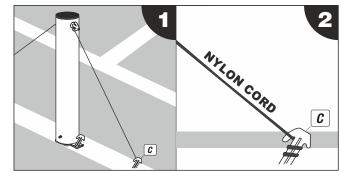
1. With your first barrier post in position use the tension peg to reinforce stability before assembling the rest of the barrier pack. Always start erecting the barrier from one side for an easy and efficient assembly (steps 1 - 2).
