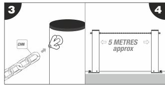
1. Attach your first chain link onto the arrowhead fitting. You will need approximately 5 metres of chain link per post distance (steps 3 - 4).
