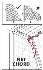
**OPTIONAL NET HOOKS** (NOT SUPPLIED WITH GOAL) MAY BE PURCHASED from itsagoal.co.uk - Easy fit net fixings can be retrofitted allowing nets to be lifted on and off with ease and fasten the net neatly to the back of the posts
