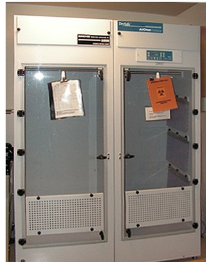
EXAMPLE 2B: Blood Drying/Wet Evidence Drying Equipment
