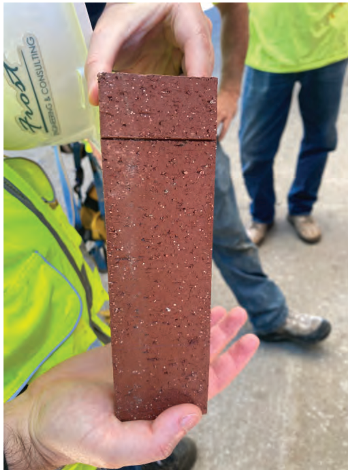
15. Bricks with deep cast marks (typical).
