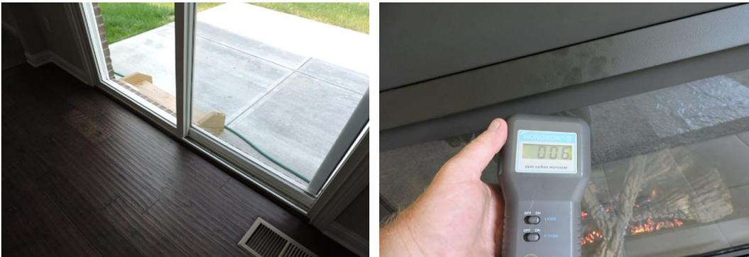
a). The **fireplace** was tested and it was functional without gas or monoxide leaks detected during operation
