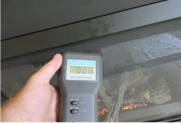
**a).** The **fireplace** was tested and it was functional without gas or monoxide leaks detected during operation
