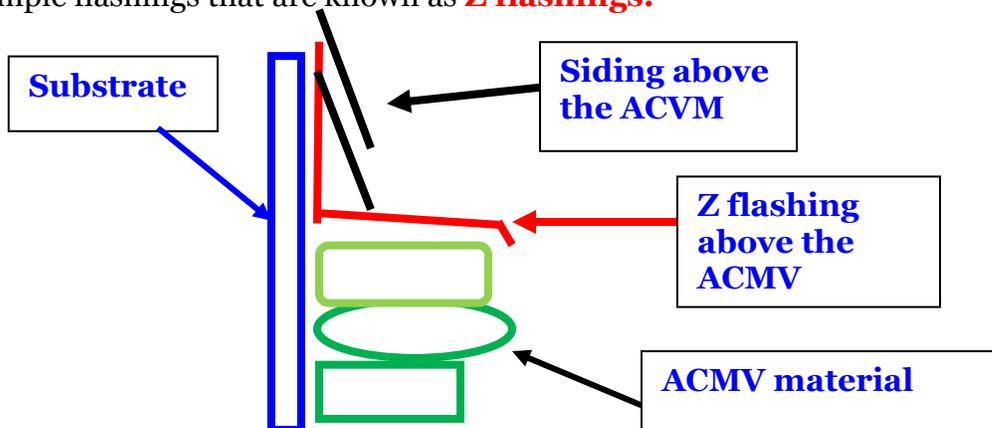
**NOTE: This drawing is intended to only show a profile of a Z flashing. There are primary and secondary materials behind the Z flashing and over the substrate that are not shown in this diagram.**
