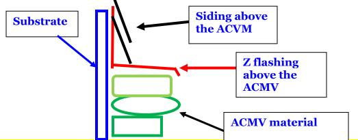
NOTE: This drawing is intended to only show a profile of a Z flashing. There are primary and secondary materials behind the Z flashing and over the substrate that are not shown in this diagram.
