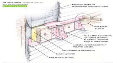
FLASHING DIVERTING WATER FROM DECK LEDGER (1 OF 2)
