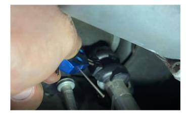
Once the clamshell clamps are removed, remove the nut retaining the AC line bracket near the strut bar mount. Remove the line bracket from the line assembly with a Phillips screwdriver.
