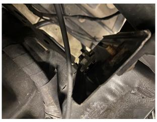
Slide the chiller bracket onto the studs so that the shelf for the chiller is pointing towards the front wheel. Place the nuts back over the studs and snug up bolts but do not fully tighten.
