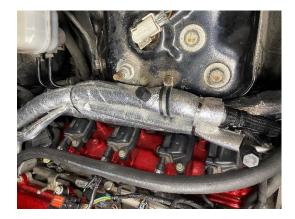
• Ensure all lines are routed to avoid the power steering pulley and any other area with moving parts.
