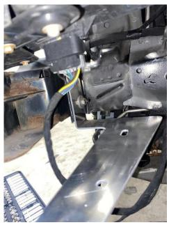
Run the AC hoses underneath the vehicle frame and in between the horns. Orient the horns so that they are not stressing the wires or connector, plug them in, and fully tighten the 10mm jam nuts.
