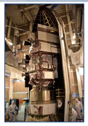
ATLAS (Laser Instrument) 550kg, Spacecraft Dry Mass 906 kg, Propellant 134 kg (7 years)
