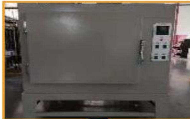
Conduct accelerated weather resistance testing on rubber materials
