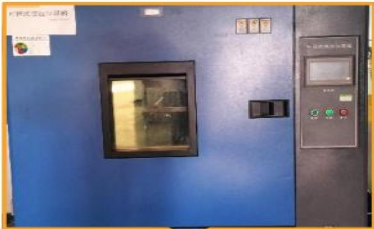
Fatigue test of air spring under simulated high and low temperature environments
