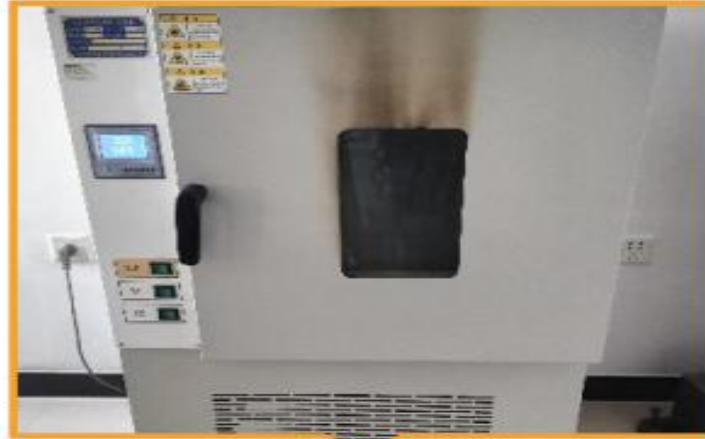
Conduct accelerated weather resistance testing on rubber materials
