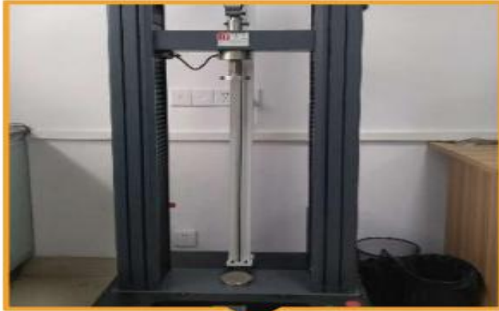
Conducting various tests to measure the tensile strength, tear strength, and elongation at break of air springs
