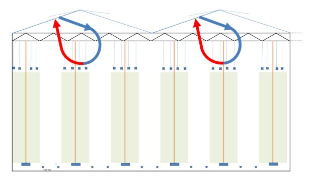
Figure 1, Airflows in a semi-closed glasshouse
