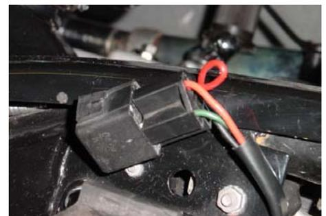
two starter relays (Standard Motor Products RY115), which plug directly into the wiring harness. If both relays “click” properly, there may be no need to remove the battery to gain access to them, as removing the battery can be quite tedious.
