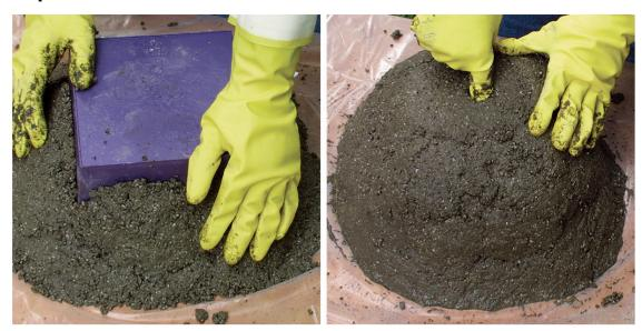
**Mold** the mixture around the chosen object, which has been placed upside down on the plastic drop cloth. Avoid objects with a pronounced lip, since it would make the object difficult to remove from the finished container.
