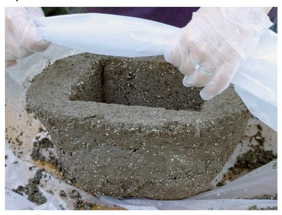
**Rewrap** your container, and place it in a shady place for another two days. Then unwrap it, and soak it with a hose periodically over the period of a few weeks to leach out the residual lime from the cement, which would harm plants.
