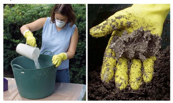
**Measure and mix** the peat moss, perlite, cement, and a small handful of reinforcing fibers in your tub. You'll kick up plenty of dust at this stage, so be sure to wear your dust mask.
