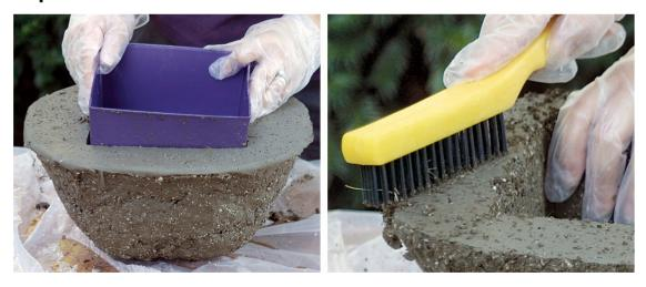
**Remove** the wrapping after the hypertufa has had a day to harden. The mixture will be firm but still soft enough to work with. Turn the container over, and remove the mold.
