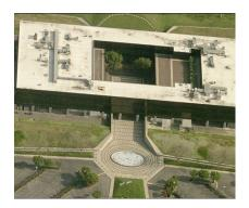
This three-story office building retrofit in Orange County features 44 NASAgrade shock absorbers. Without this innovative technology, it would not be financially feasible to seismically strengthen this circa 1969, steel and concrete building. Miyamoto determined that fluid viscous dampers, which NASA and the U.S. military use to dissipate seismic energy, can
