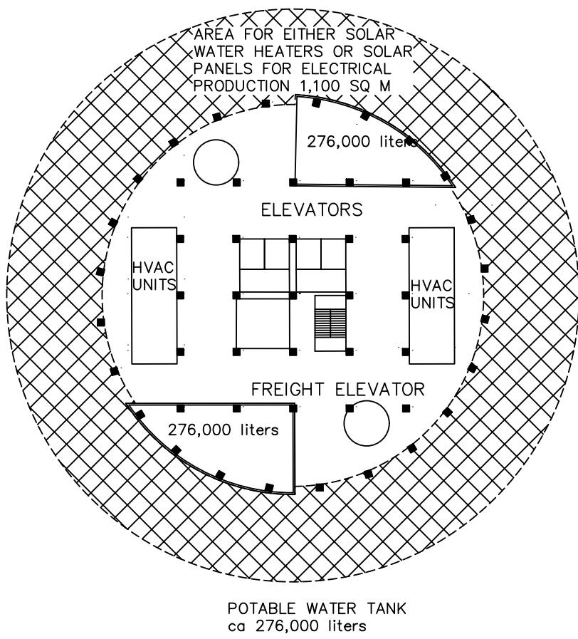
THE 15TH OR TOP FLOOR HERE ARE ELEVATOR SERVICE CUBES. HVAC UNITS TWO POTABLE WATER TANKS, TWO VERTICAL AXIS WIND TURBINES AND 1,100 SQUARE METER AREA FOR EITHER SOLAR WATER HEATERS OR SOLAR PANELS WHICH EVER IS THE MOST EFFICIENT USE OF THE AREA. AT THIS STAGE NOT SURE HOW MUCH POWER THE VERTICAL AXIS WIND TURBINES CAN GENERATE.
