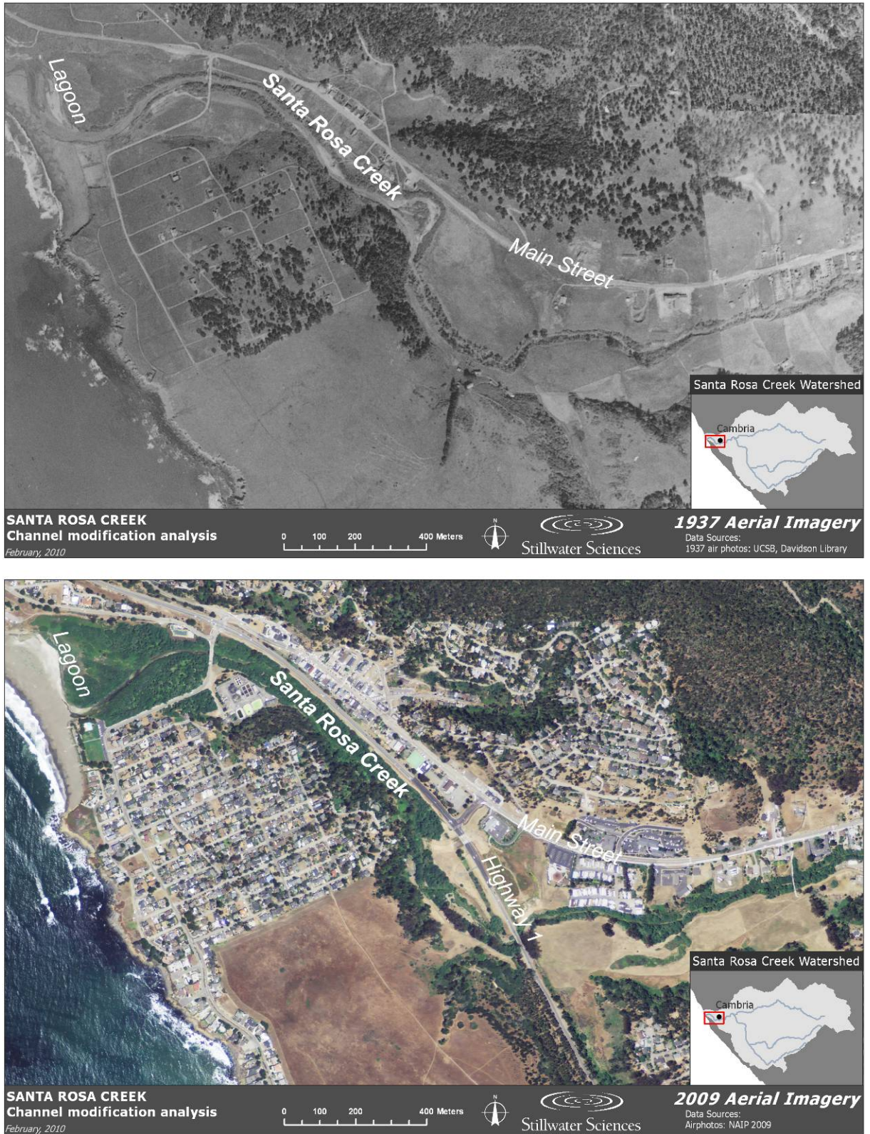
Figure 4-16. Historical (1937) and current (2009) aerial photographs showing the Lower reach of Santa Rosa Creek near the town of Cambria.
