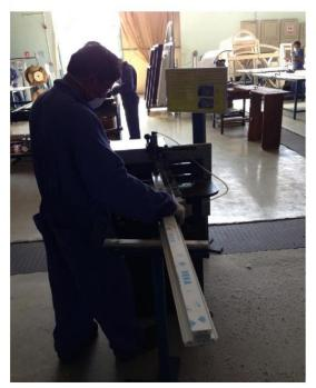
8. ARCH BENDING Machine - for making arch profiles / for bending
