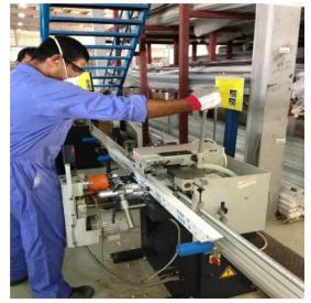
**4. REINFORCEMENT SCREWING MACHINE** – For screwing reinforcements to Profile
