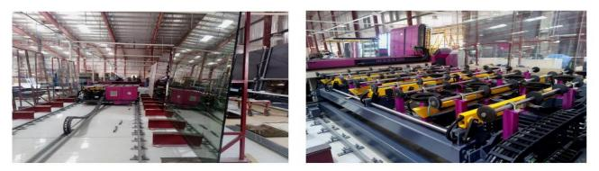
**2. CNC GLASS CUTTING Machine** – Glass sheets are loaded onto the Cutting table. The glass sizes are optimized on the CNC machine to minimize wastage and the glass is cut to desired sizes.
