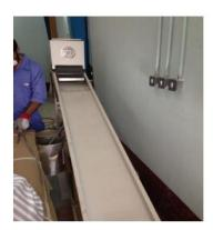
**4. BUTYL Extruder Machine** – Machine applies Butyl on either side of the spacer bar to fix it firmly onto the two glass panes on either sides in order to proceed for the double glazing process.
