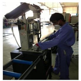
**5. DOUBLE HEAD Welding Machine** – For welding the adjacent uPVC Profiles after screwing the reinforcements to UPVC Profile
