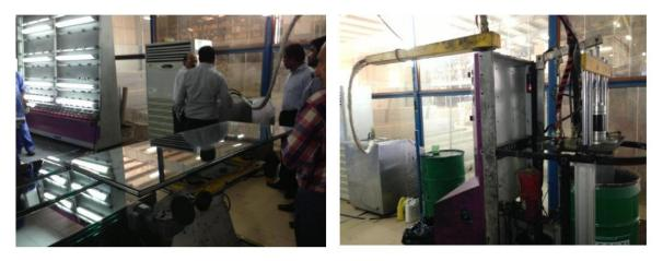
6. VERTICAL Panel PRESSING UNIT + AUTOMATIC GLASS Sealing Robot - Automatic glass sealing robot carries out the final sealing of the insulating glass units, providing accurate sealing of the angles and assuring high operating speed.
