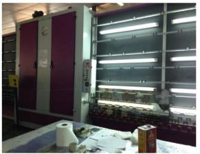
**3. DESSICANT Filler Machine** – This machine fills desiccant molecules inside the spacer bars in the 12mm airspace between the two 6mm glass panes on either sides of the spacer bar. Desiccant molecules absorb any moisture.
