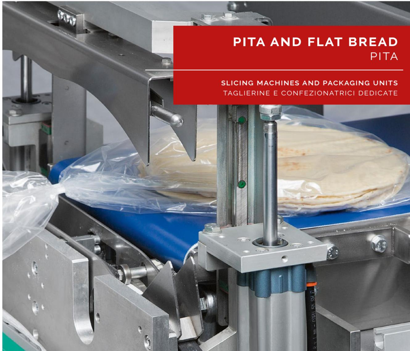
Not only packaging, but also slicing. This products can be fully or partially sliced and packed in preformed bags with sealing if required or on flow-pack for a complete closed and sealed pack.
