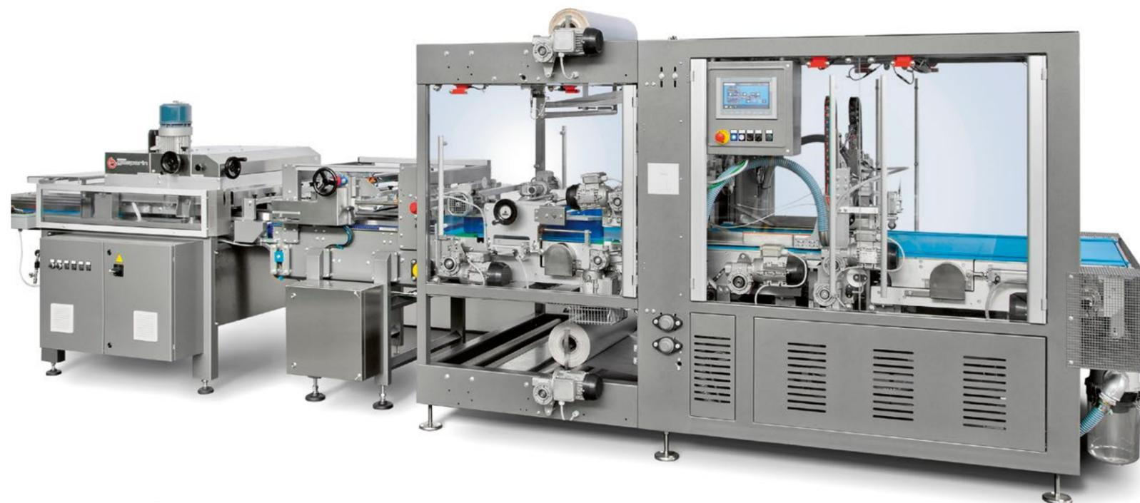
Automatic slicing and packaging lines for buns, baguettes, bagels and bakery products used in fast food sector. The slicing of these products can be total or partial. Packaging can be flow-wrapping type, in bags or in Bulk-packer in order to ensure a complete range of solutions to meet different production needs.
