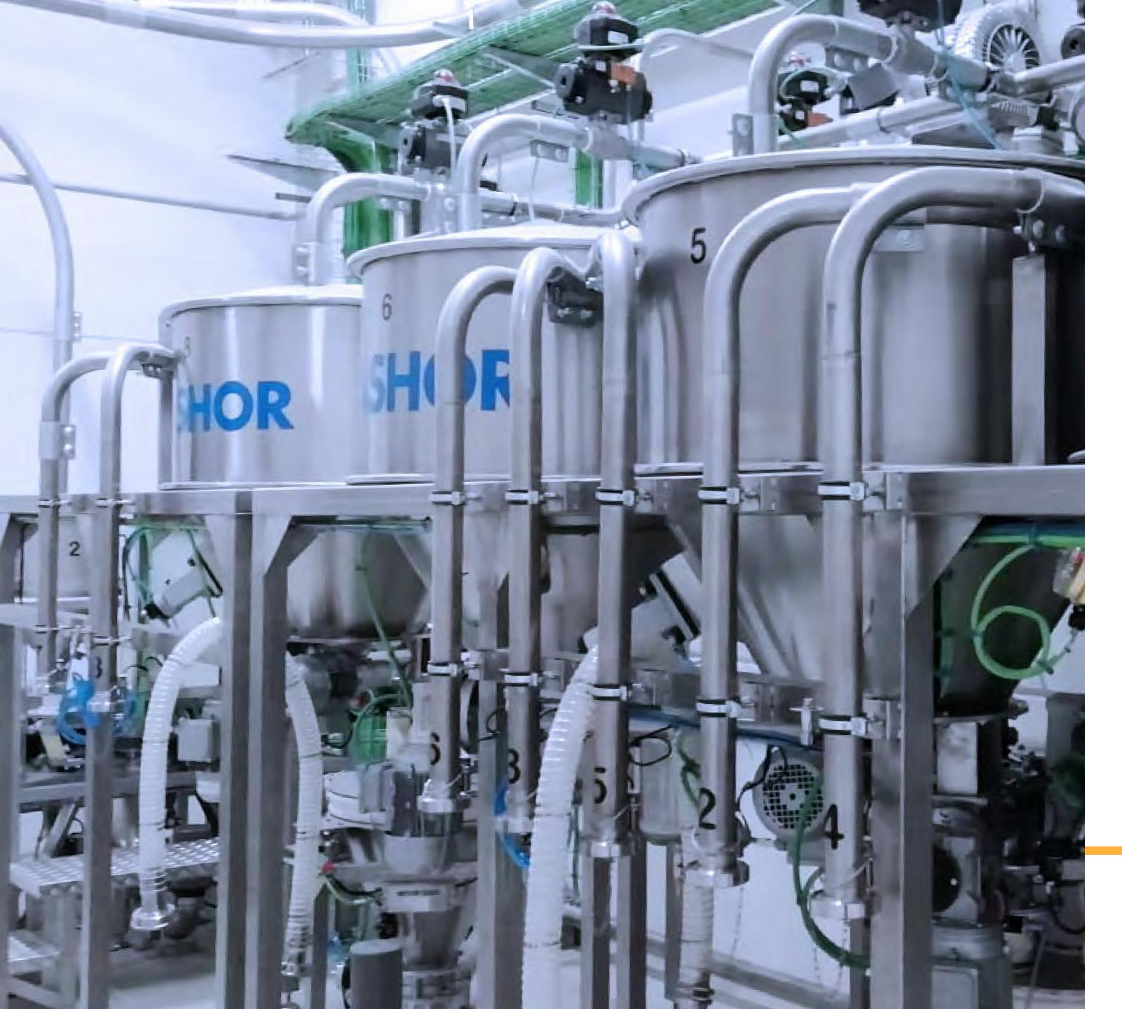
We have micro-dosage stations for solids and liquids. The stations can also be semi- or fully automatic.
