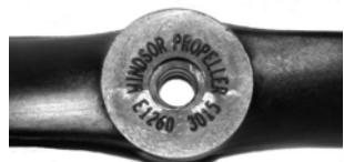
Most Master Airscrew Propellers have two hole sizes because they are piloted in the back of the propeller to facilitate reaming should you need to enlarge the hole. The first number is the hole size; second number is the pilot size.
