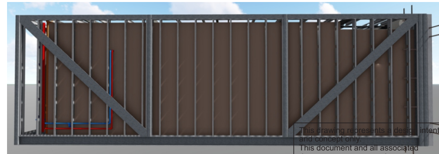
GALVANIZED METAL SHEETROCK CEILING STUDS WITH ACOUSTICAL INSULATION
