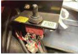
1. Flip the power switch lever to the "RUN" position to turn on the power supply of the complete vehicle.
