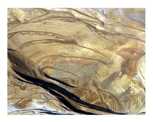
Aerial photo of the Round Mountain open pit mine. In 2008 the dimensions of the pit were about 8,200 feet by 4,900 feet, it has grown since that time. The mining benches (contour lines) are each about 35 feet high so you can see that this is a big hole.
