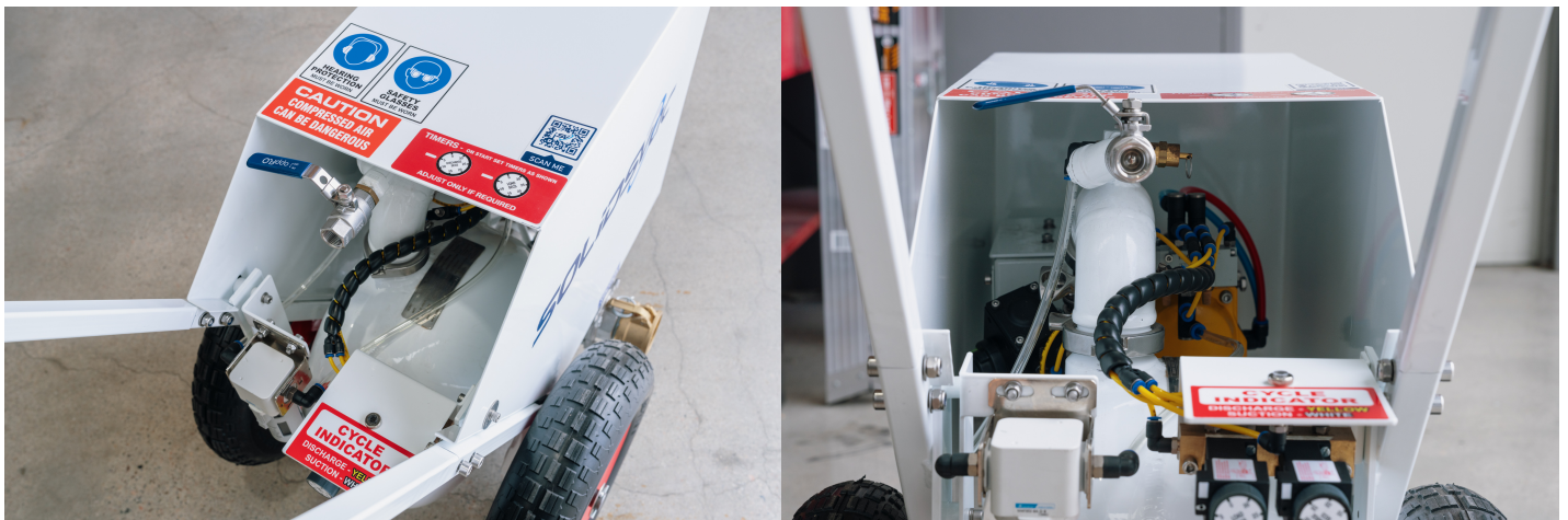
SV20-SP Pneumatic Control Items (Pressure Gauge, Cycle Indicator and Adjustable Timers)
