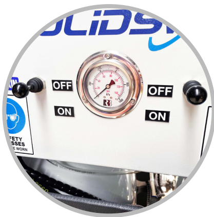
CONTROL BOX NEUTRAL POSITION
