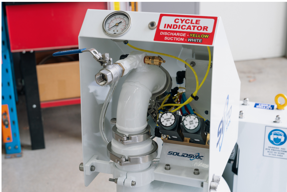
SV100-SPDK Pneumatic Control Items (Pressure Gauge, Cycle Indicator and Adjustable Timers)
