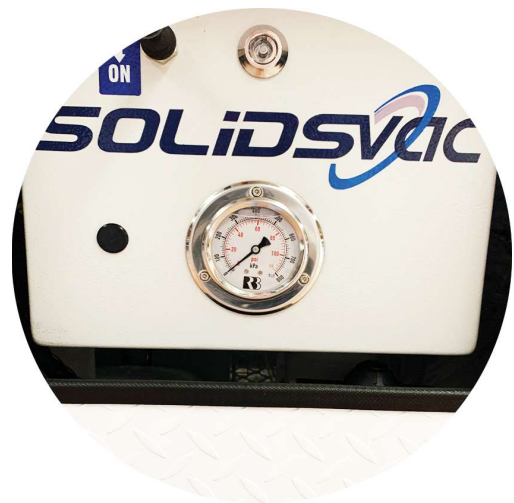
Operational pressure gauge
