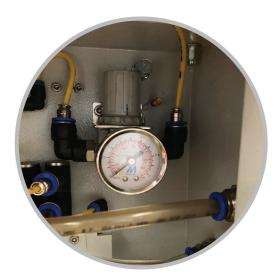
PNEUMATIC CONTROLS PRESSURE GAUGE WITH REGULATOR
