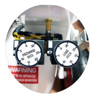
Adjust timers to dial marking beside each timer. Only adjust timers when required.
