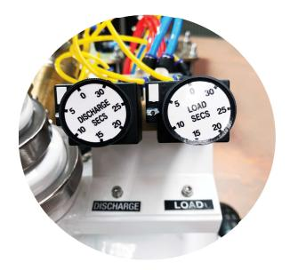
Adjust timers to dial marking beside each timer. Only adjust timers when required.
