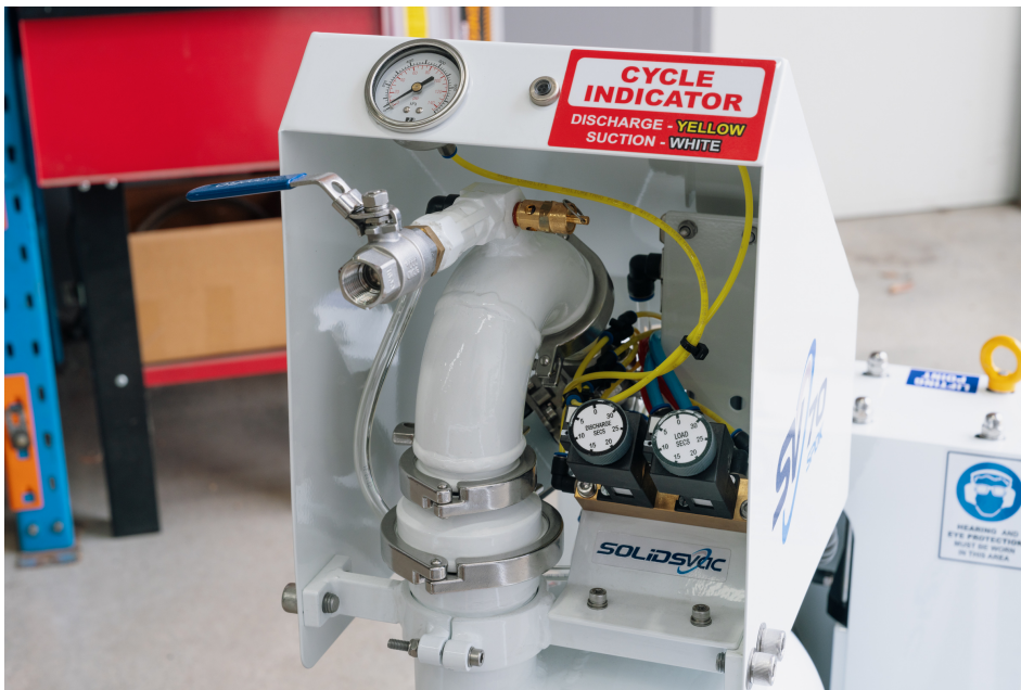
SV70-SPDK Pneumatic Control Items (Pressure Gauge, Cycle Indicator and Adjustable Timers)
