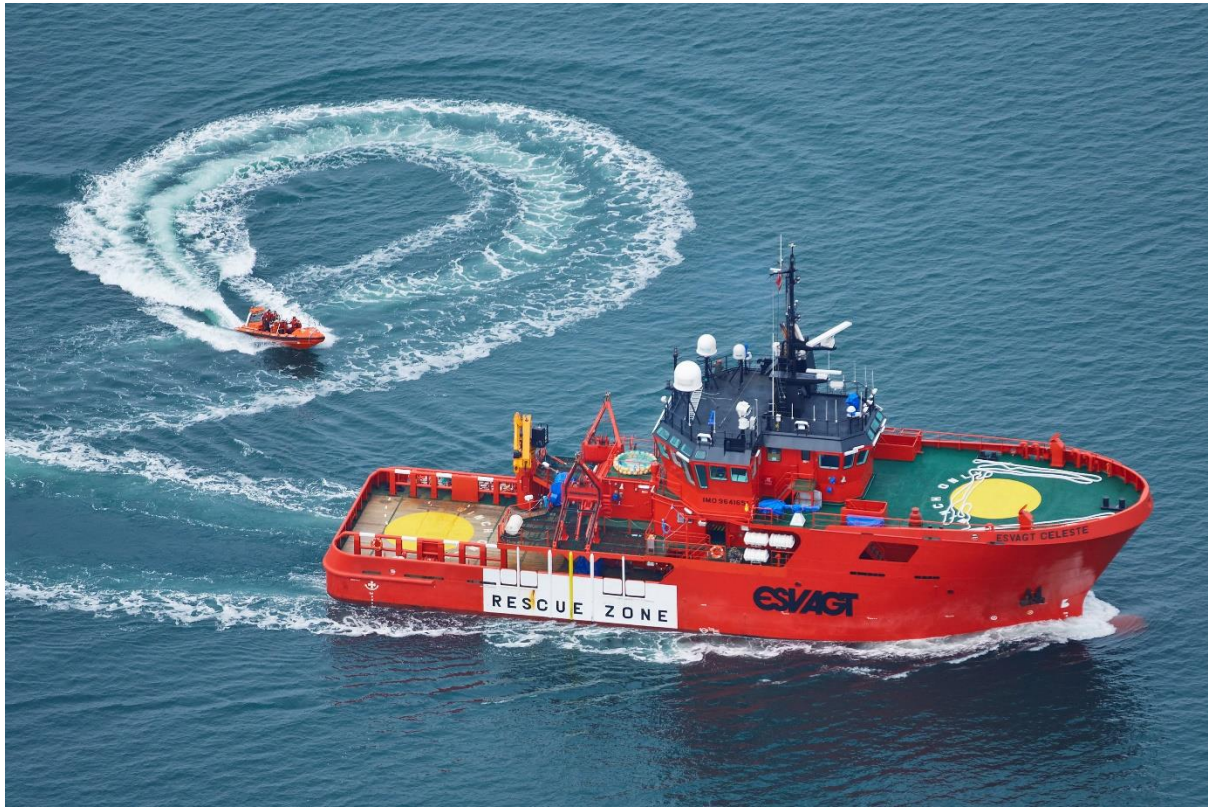
Above: A standard ERRV with high-speed daughter craft and high levels of mass casualty equipment, SAR capability and medical facilities
