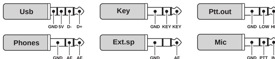
Ptt.out, LOW: low level on transmit, HI: high level on transmit.
