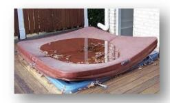
Sometimes a hot tubs cover which has been weight-stressed will develop water puddles due to sagging. Some cheap covers (as well as older ones) were not designed with a tapered core for proper water runoff, which exacerbates the problem. If you start to get a small puddle on your cover, unzip the vinyl covering and carefully remove the foam core, then flip it over. Flipping it sometimes corrects the issue (at least temporarily) if not too severe.
