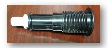
The drain plug, pictured above, allow you to drain your hot tub of water. It works by twisting the Drain Plug Water Hose Adapter onto your water hose. Screw the Drain Plug Hose Adapter into the Drain Plug and the water will flow out of the water hose
