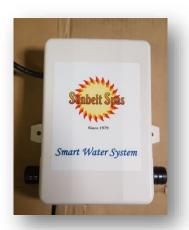
**Ozonator** – The Ozonator, long black tube or white rectangular box pictured above, produces O3 molecules that are released into the water. These molecules enter the spa water through the ozone injector jet and help to kill bacteria and most unicellular microorganisms. This option helps you maintain your Sunbelt Spa and utilize fewer chemicals. The Ozonator will operate each time the spa filtration functions are in service.
