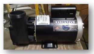
The water pump pictured here pushes the water from the spa through your jets. Pumps operate through the spa pack ( ) button and have two speeds.
