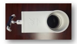
The shut off valve is a slice valve that stops water flow from the pump to the attached pipes. In the up position the slice valve allows for complete water flow and spa operation. In the down position the slice valve closes and the water is stopped from flowing. These slice valves allow a spa technician to remove the pump and replace the pump without having to empty all of the spa water.
