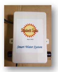
The Ozonator, long black tube or white rectangular box pictured above, produces O3 molecules that are released into the water. These molecules enter the spa water through the ozone injector jet and help to kill bacteria and most unicellular microorganisms. This option helps you maintain your Sunbelt Spa and utilize fewer chemicals. The Ozonator will operate each time the spa filtration functions are in service.
