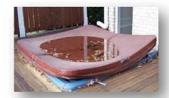
Sometimes a hot tubs cover which has been weight-stressed will develop water puddles due to sagging. Some cheap covers (as well as older ones) were not designed with a tapered core for proper water runoff, which exacerbates the problem. If you start to get a small puddle on your cover, unzip the vinyl covering and carefully remove the foam core, then flip it over. Flipping it sometimes corrects the issue (at least temporarily) if not too severe.
