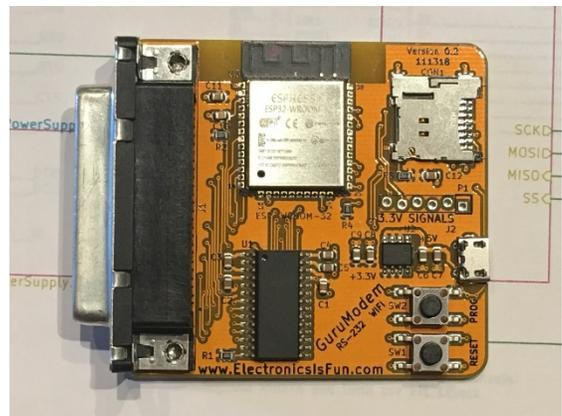
The GuruModem connects easily to the computer's serial port either directly or over a serial cable. Power must be supplied to the board from a +5V power adapter with a micro USB connector (similar to the power adapters used for the Raspberry Pi). The computer can communicate with the GuruModem over a standard RS-232 serial interface at speeds up to 230.4K baud\* with the appropriate software and cable. The maximum speed is dependent on the computer hardware and software.
