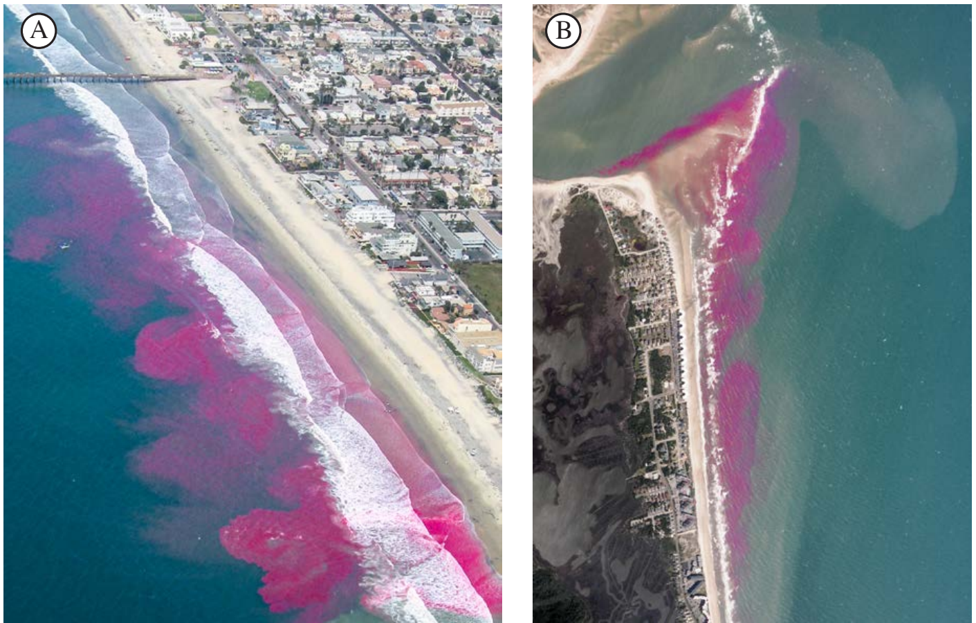
Figure 6: Photographs of non-toxic fluorescent dye tracer (pink water) (a) one hour after continual surfzone dye release begins at Imperial Beach California (Hally-Rosendahl et al. 2014), and (b) 1.5 hours after continual tidal inlet dye release during ebb tidal flow at New River Inlet, North Carolina. In both cases, dye serves as a mock pollutant and study of its transport and dilution will inform how pollutants from pathogens to chemical contaminants evolve in nearshore waters. (image from Clark et al. 2014).
