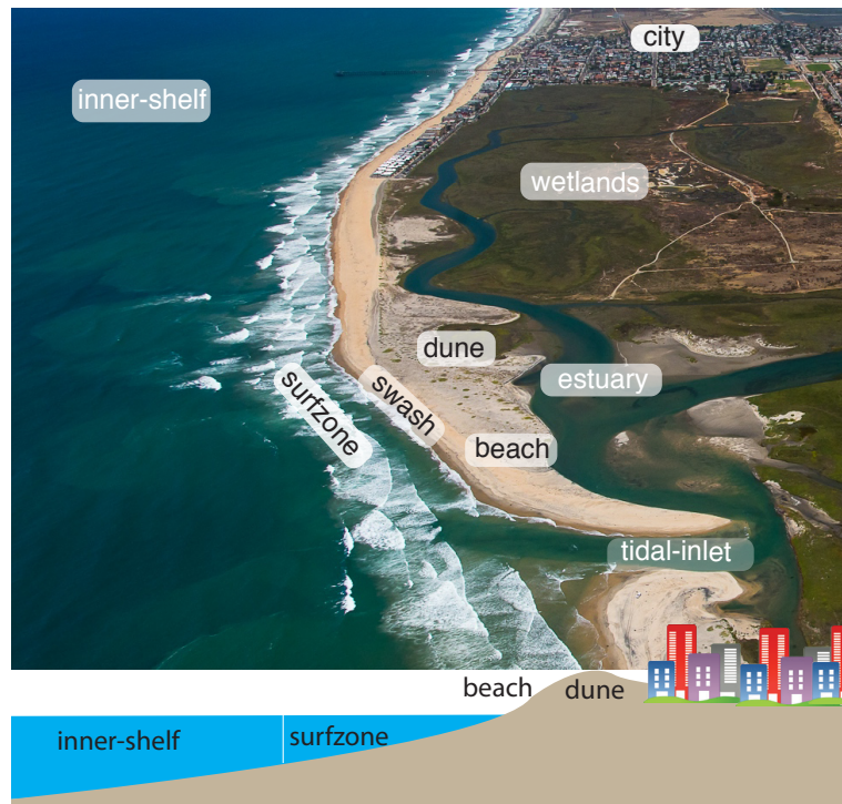
Figure ES-1. (top) Nearshore region schematic including the inner-shelf, surfzone, swash, beach, dunes, tidal-inlet, estuary, and city in a coastal plain. (bottom) Idealized cross-shore profile of the nearshore.
