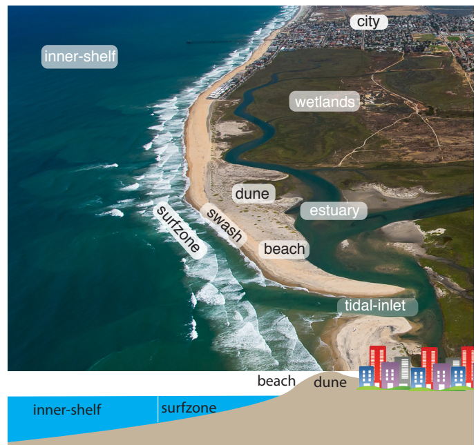
Figure 1. (top) Nearshore region schematic including the inner-shelf, surfzone, swash, beach, dunes, tidal-inlet, estuary, and city in a coastal plain. (bottom) Idealized cross-shore profile of the nearshore.
