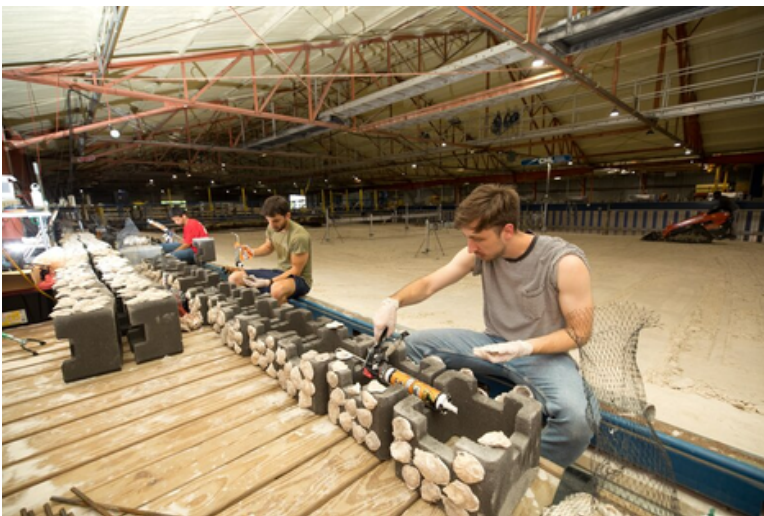
(Left) Researchers building a representative “oyster reef” in the large wave basin, and (right) a group of researchers from several universities collaborating in the wave flume at ERDC-CHL during SEDCOLAB.
