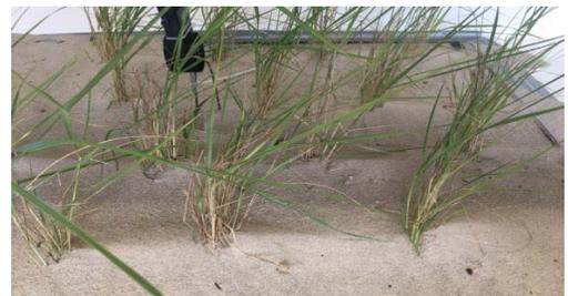
**Left:** The wind tunnel which has a 1m x 1m moveable bed test area where boxes established with plants can be inserted. **Right:** *A. breviligulata* plants at 6-inch spacing and the resulting bedforms built around their base post-experimental trial.
