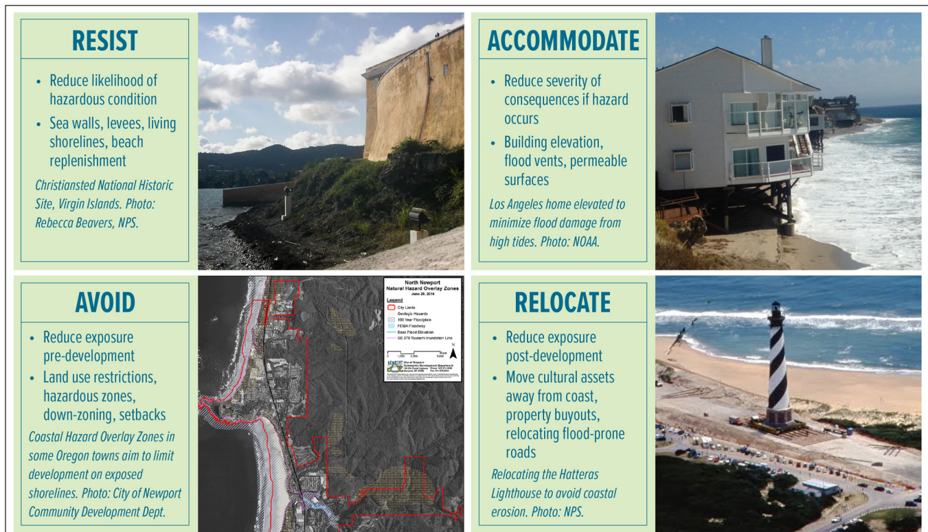
Figure 8. Examples of coastal adaptation strategies — resist, accommodate, avoid, or relocate (Doberstein et al. 2018) — and representative infrastructure and management sites. Images are reproduced with permission from (upper left) U.S. National Park Service (2019), Seawalls, Bulkheads, and Revetments; (upper right) NOAA National Ocean Service (2021); (lower left) City of Newport Community Development Department (2016); (lower right) U.S. National Park Service (n.d.), Cape Hatteras Light Station. Complete citations appear in the reference list.
