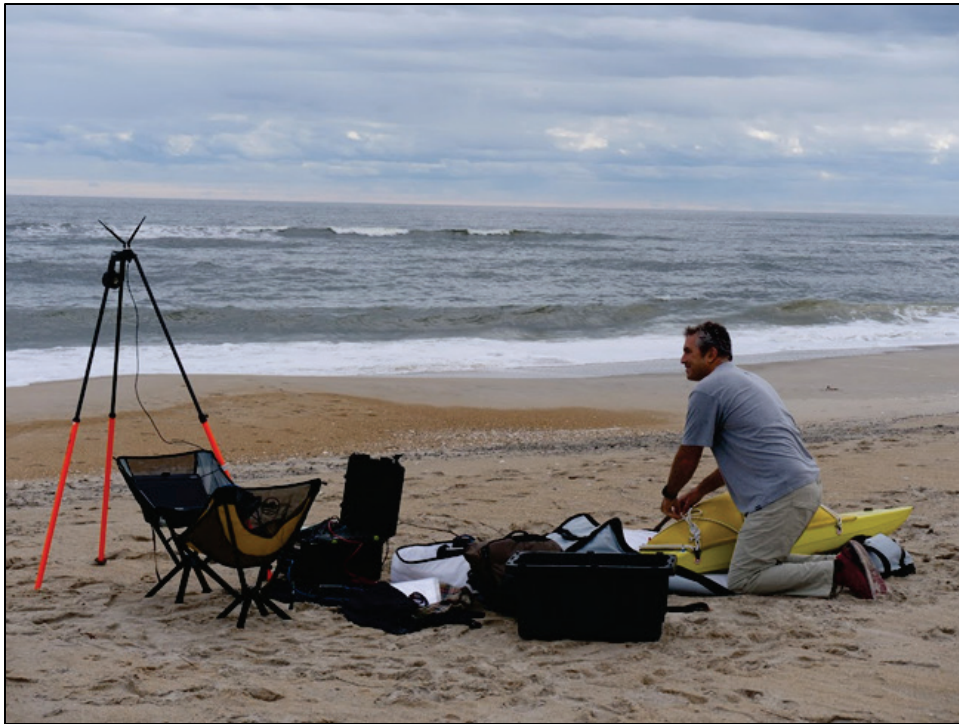
Figure C-14. Traykovski preparing one of his unmanned autonomous surface vehicles to measure bathymetry at the southern DUNEX site (photo credit: Sherwood, date unknown).
