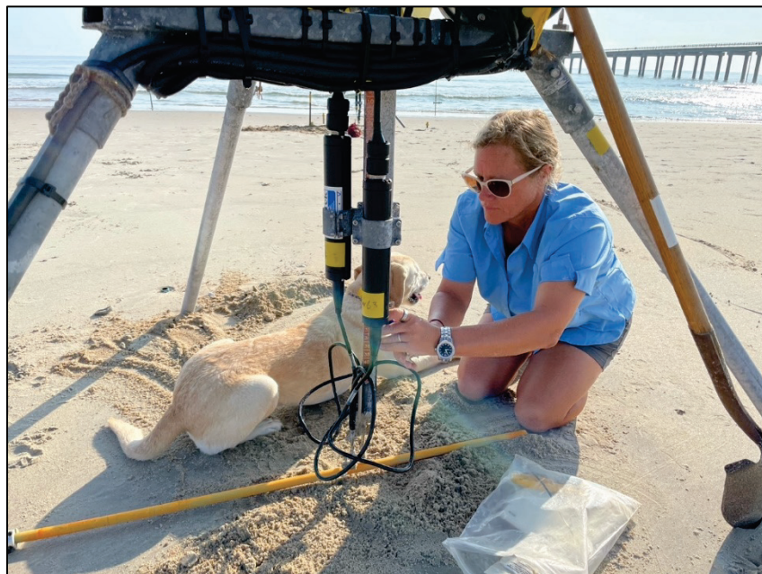
Figure C-4. Raubenheimer and guide dog Hugger adjust vertical elevations of swash velocimeters mounted on a tripod on the beach north of the FRF pier (photo credit: Elgar).
