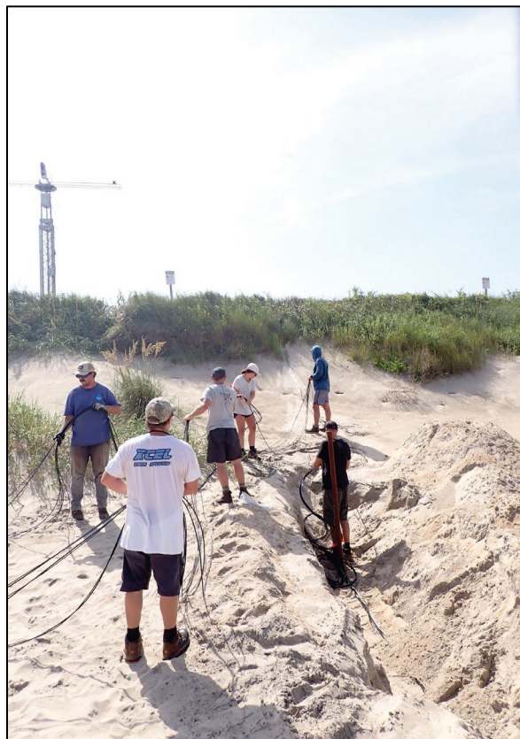
Figure C-3. Swash array installation of in situ pressure sensors and velocimeters at the FRF in Duck, North Carolina.
