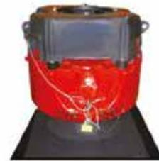
CASING SPIDER/ELEVATOR 350 TON
