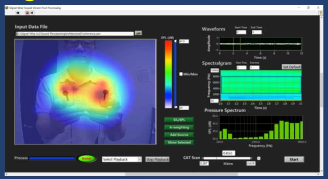
Two earphones emitting the <u>coherent broadband</u> sounds that were generated by the same laptop computer were located. The separation distance between these earphones was less than 20 cm, much shorter than the wavelengths of the sound waves.
