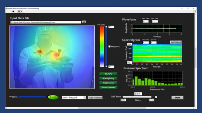
Two earphones emitting the <u>coherent narrow-band</u> sounds that were generated by the same laptop computer were located. The separation distance between these earphones was less than 20 cm, much shorter than the wavelengths of the sound waves.
