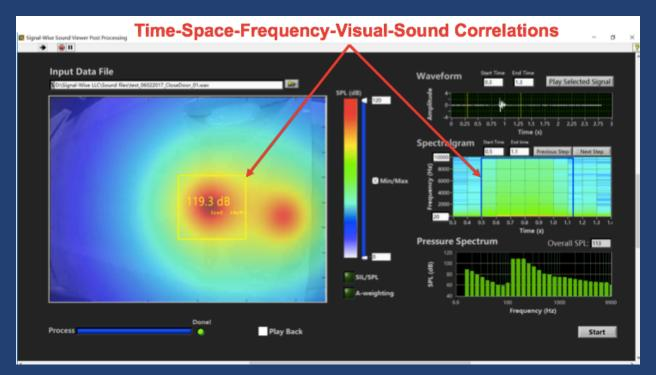
Sound Viewer enables one to analyze transient door slamming sounds and correlate time-space-frequency-visual-audio relationships by visualizing the acoustic pressure distribution over the entire frequency range from 20-20,000 Hz. It also allows users to estimate the acoustic power, namely, source strengths at user-defined areas of these transient sounds.
