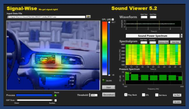
Sound Viewer enables one to locate HVAC noise with the fan running at the lowest speed, which was barely noticeable, while the engine was running at the idle speed.
