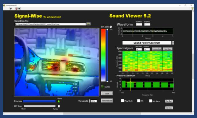
Similarly, Sound Viewer enables one to locate HVAC noise with the fan running at the highest speed, which was very noisy, while the engine was running at the idle speed.
